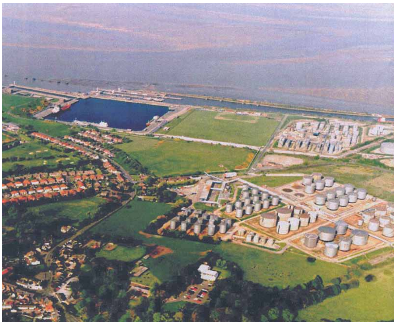
Figure 15 Site layout showing the location of the two bulk tank storage facilities and the adjacent dock from where deliveries by ship are made
